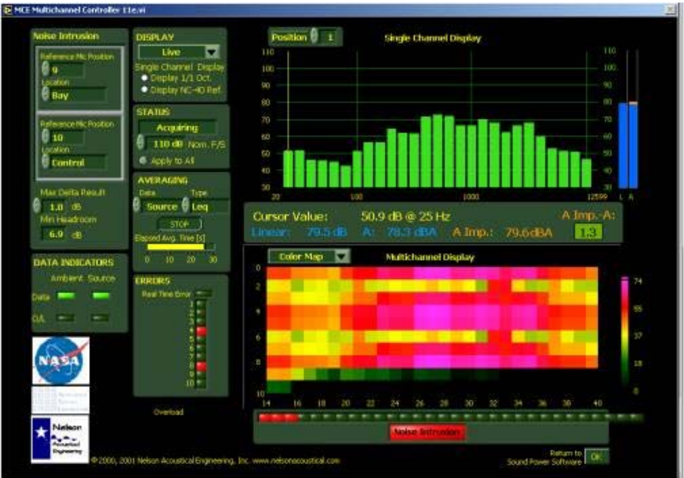
Figure 4 – Screen shot from multi-channel real time analysis display of ATL custom data acquisition system software. Noise Intrusion Alarm indicator shows bands which may have been affected by external noise during the acquisition.
